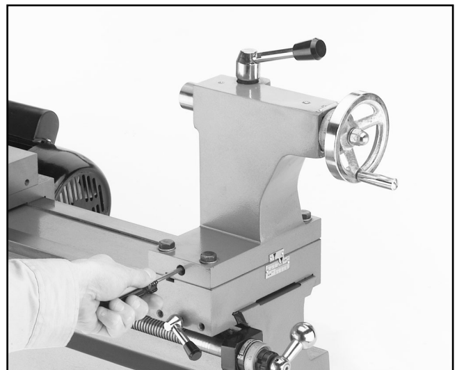
Figure 36. Tailstock offset adjustment screw.
